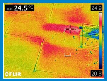
Figure 3.5: Thermal Fault Hotspot
