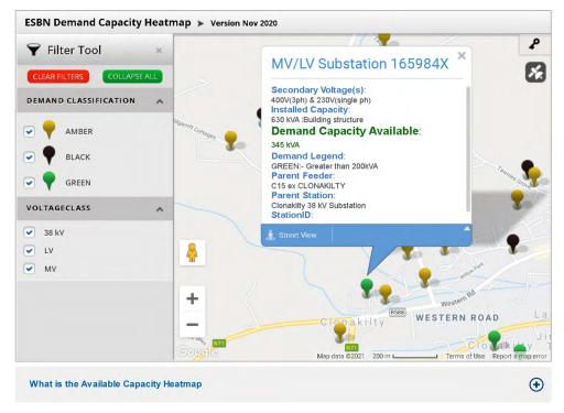
Figure 4.2: Demand Heatmap Layout Showing Voltage and Marker Filter Options
